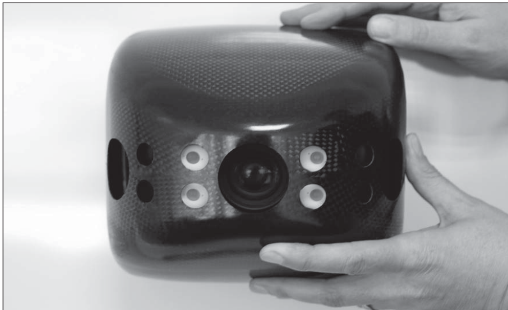
The 3D camera in the flying robot can identify small objects measuring 20 by 15 centimeters from seven meters away. (© Fraunhofer IMS) | Picture in color and printing quality: www.fraunhofer.de/press
