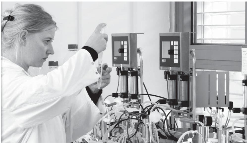
The researcher takes samples from the bioreactor. (© Fraunhofer IGB/Frank Kleinbach) | Picture in color and printing quality: [www.fraunhofer.de/press](http://www.fraunhofer.de/press)
