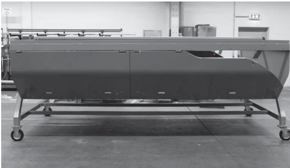
**Although this diesel engine housing for trains is made of a light polyurethane-based material, it is nonetheless capable of withstanding extreme stresses. (© Fraunhofer ICT) | Picture in color and printing quality: [www.fraunhofer.de/press](http://www.fraunhofer.de/press)**
