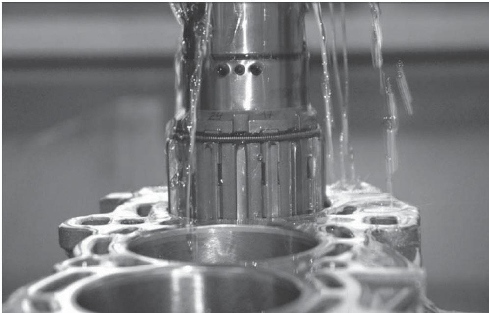
The honing tool adjusts its shape to match the piston bore holes. (© Fraunhofer IWU) | Picture in color and printing quality: [www.fraunhofer.de/press](http://www.fraunhofer.de/press)
