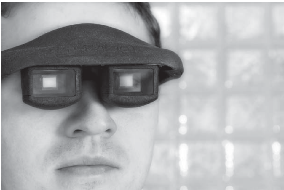
Users can control the display of these data glasses with their eye movements. (© Fraunhofer COMEDD) | Picture in color and printing quality: www.fraunhofer.de/press
