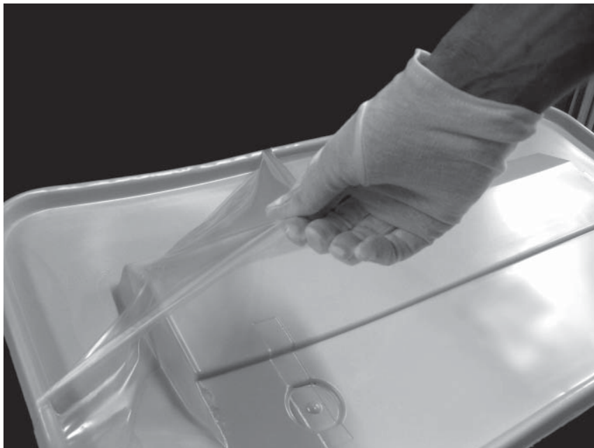
Release from mold, transfer and protection with Flex PLAS ® technology from Fraunhofer IFAM. (© Fraunhofer IFAM) | Picture in color and printing quality: www.fraunhofer.de/press
