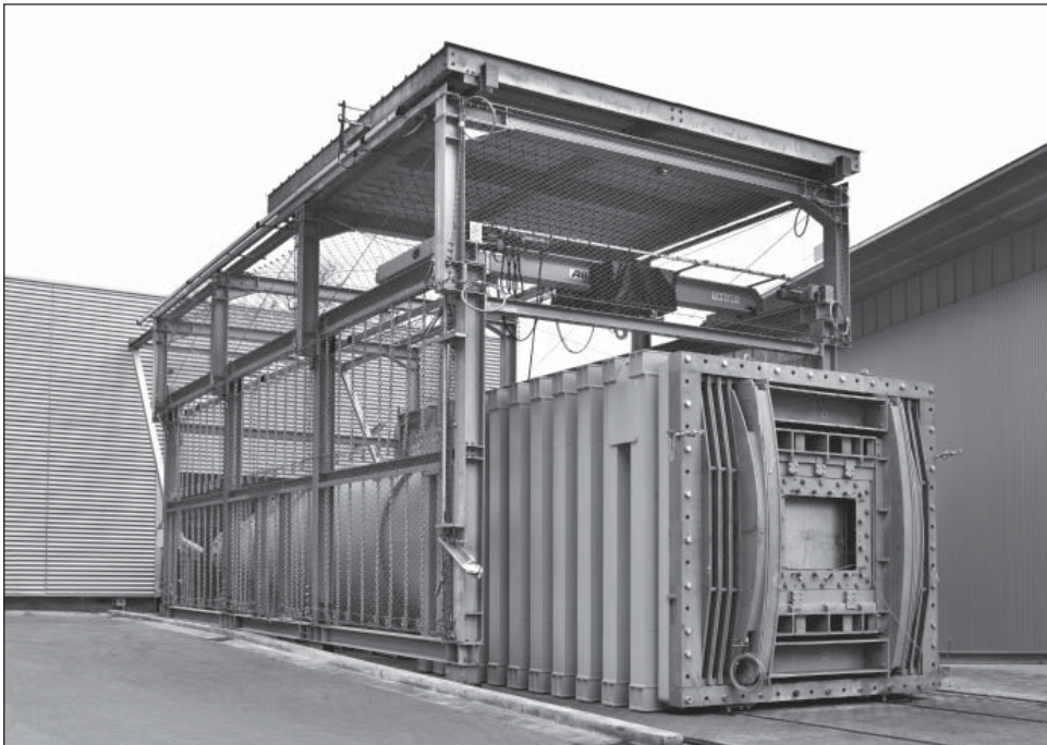
Researchers use this apparatus to identify the stresses at which windows and glass facades crack and shatter. (© Fraunhofer EMI) | Picture in color and printing quality: www.fraunhofer.de/press
