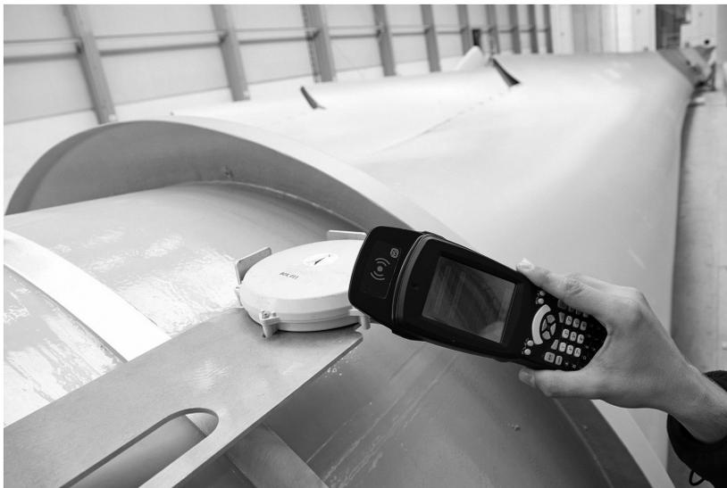
RFID chips in the module and in the locator make automatic continuous tracking possible.
