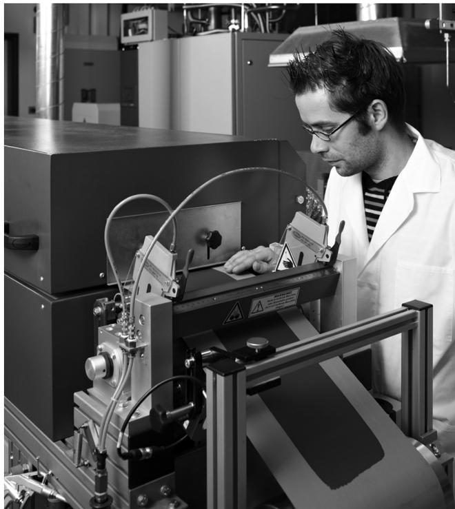
**Roll-to-roll coating of electrodes at IWS: The scientists now have optimized the design of anode and cathode for lithium-sulfur batteries. (© Jürgen Leibmann) | Picture in color and printing quality: [www.fraunhofer.de/press](http://www.fraunhofer.de/press)**
