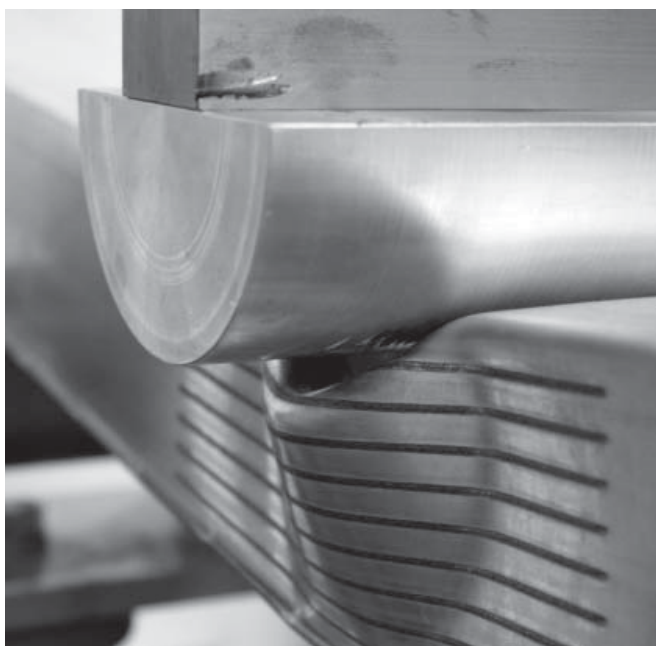
This crash test is designed to establish how much a sample component deforms under a defined bending stress. (© Fraunhofer IWS) | Picture in color and printing quality: www.fraunhofer.de/press
