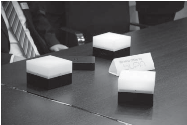
These office lamps are powered cordlessly. (© Fraunhofer ENAS) | Picture in color and printing quality: www.fraunhofer.de/press
