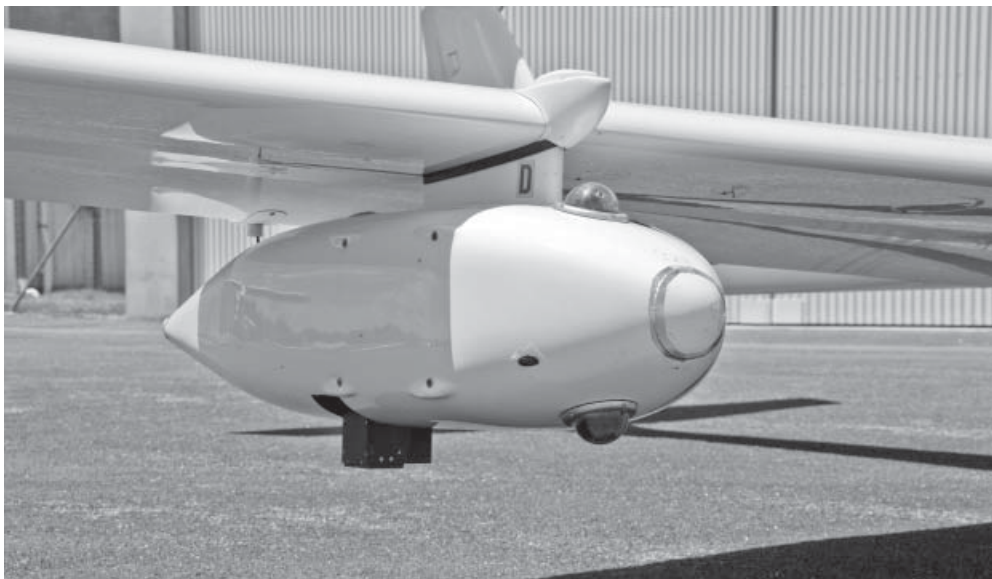
The hyperspectral camera is mounted under the wing of the airplane used for research. (© Fraunhofer IFF) | Picture in color and printing quality: www.fraunhofer.de/press
