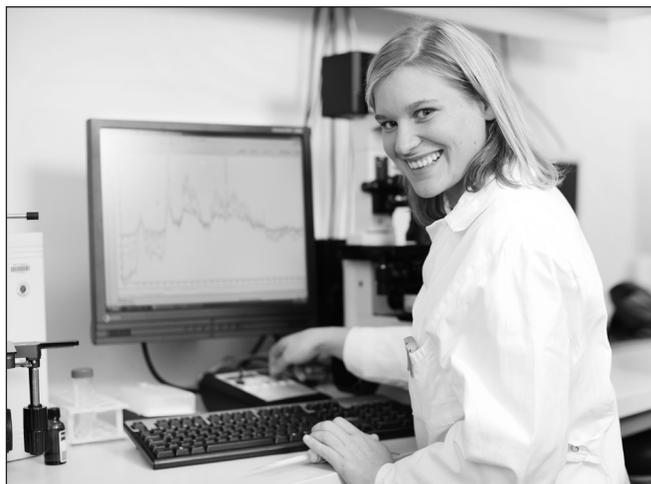
**The optical analysis system of IGB: the spectra recorded by the Raman spectroscope (back right) are displayed graphically on a monitor screen. The scientist controls the laser with the small box. (© Fraunhofer IGB) | Picture in color and printing quality: [www.fraunhofer.de/press](http://www.fraunhofer.de/press)**
