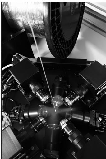
**With the WIRE-AOI wire inspection system, four cameras collectively deliver 40,000 analyzed images per second. Thus, a 100% control of the wire surface in real time can also work with very rapid production processes. (© Fraunhofer IPM) | Picture in color and printing quality: [www.fraunhofer.de/press](http://www.fraunhofer.de/press)**
