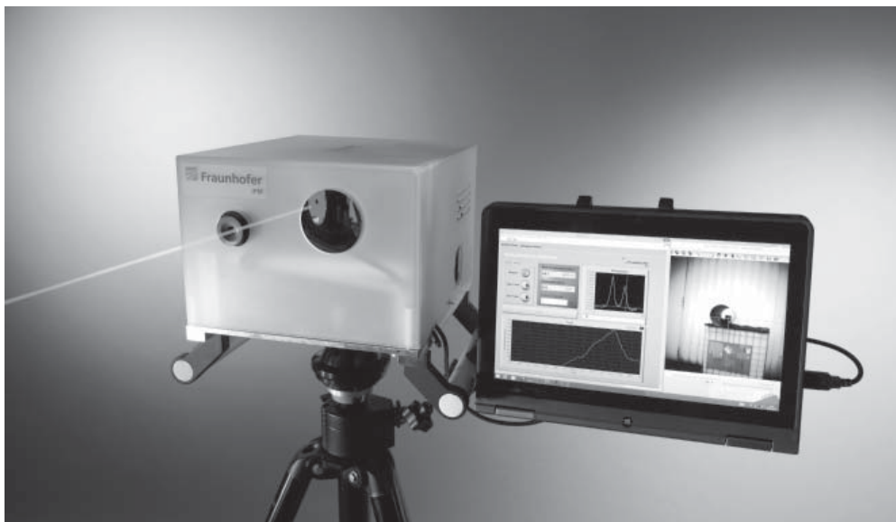
The laser-based system measures escaping biogas without contact – even from several meters away. (© Fraunhofer IPM) | Picture in color and printing quality: www.fraunhofer.de/press
