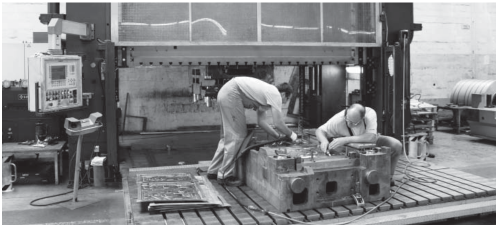
Trained workers at Gorenje install sensors in the tool components of a press used to produce parts for household appliances. (© Gorenje Group) | Picture in color and printing quality: www.fraunhofer.de/press
