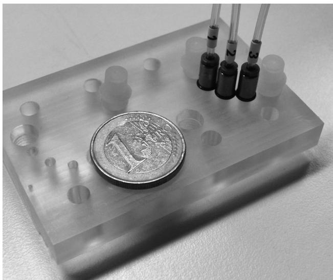
**Using the compact multi-organ chip (comparable in size to a one-euro piece), and those of three separate microcircuits, researchers can study the regeneration of certain kidney cells (© Fraunhofer IWS) | Picture in color and printing quality: [www.fraunhofer.de/press](http://www.fraunhofer.de/press)**
