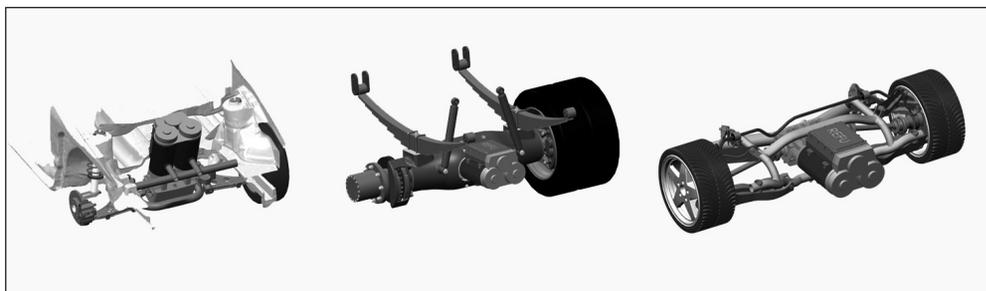
**In electric commercial vehicles of the future, the drive will be integrated into the axle. Modules consisting of a drive and axle are scalable for various vehicle types. (© Fraunhofer IWU) | Picture in color and printing quality: [www.fraunhofer.de/press](http://www.fraunhofer.de/press)**
