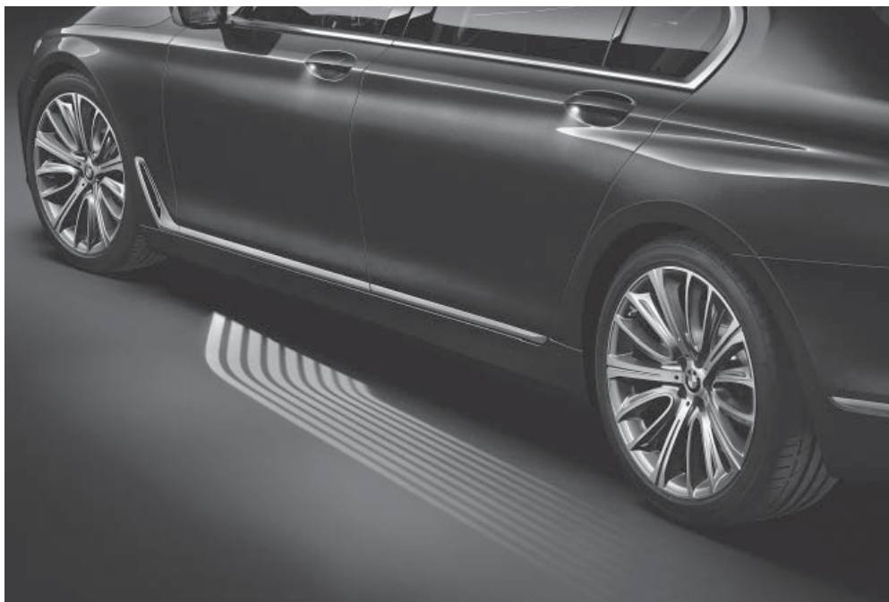
Microlenses project light onto the entry area of the new BMW 7 Series. (© BMW) | Picture in color and printing quality: www.fraunhofer.de/press
