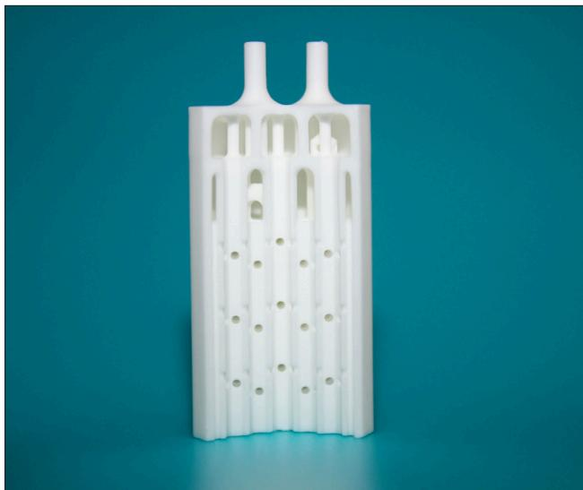
**Cut through a ceramic microreactor which was manufactured additively: the complex channels as well as the fluidic connections at the top were printed together with the whole component.**
