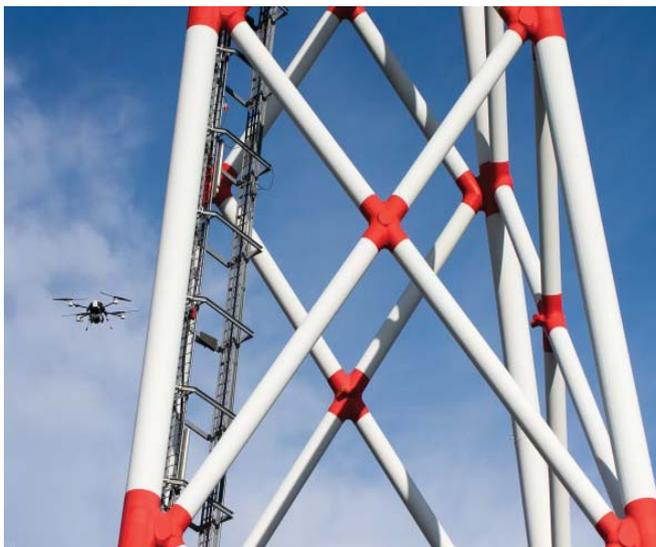
A drone being used to inspect an offshore wind turbine.
