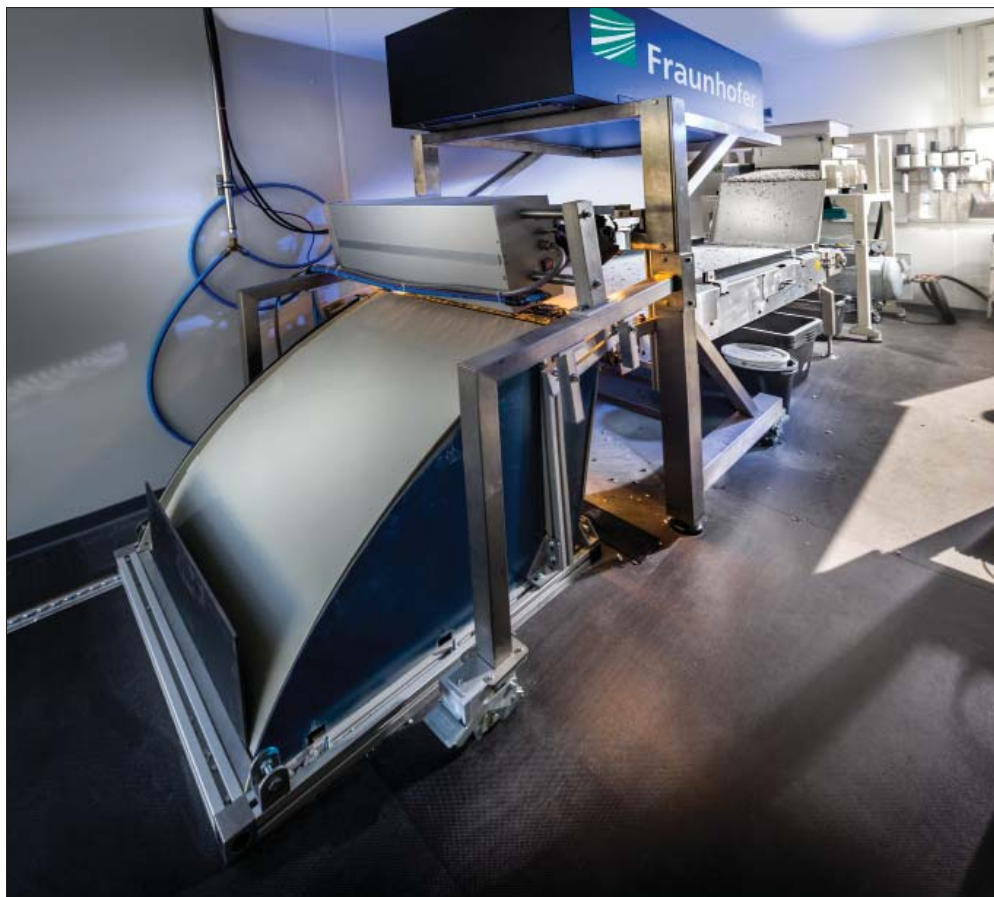
Sorting machine with conveyor belt, which transports the shredded plastic waste. © Fraunhofer IOSB | Picture in color and printing quality: www.fraunhofer.de/en/press .
