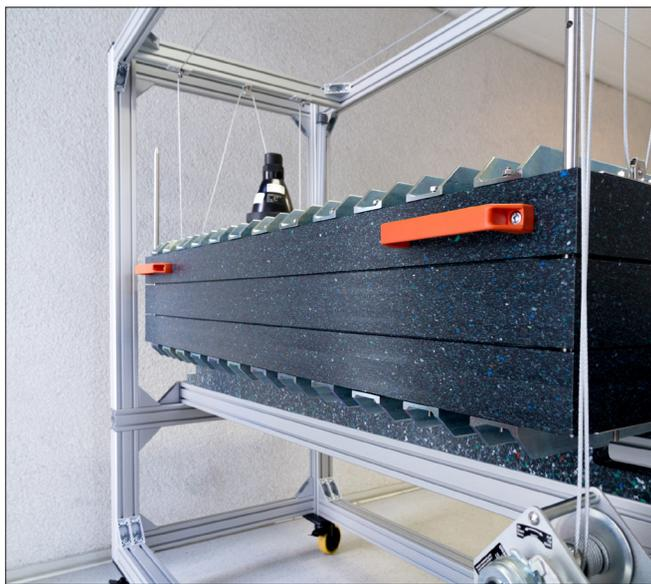
The electrolysis cell ePhos® extracts nitrogen and phosphorus purely electrochemical. The process is very straightforward and doesn't require to stock chemicals. © Fraunhofer IGB | Picture in color and printing quality: [www.fraunhofer.de/en/press](http://www.fraunhofer.de/en/press)
