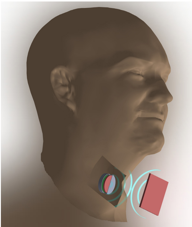
Basic structure of ultrasound power supply and communication. © Fraunhofer IBMT | Picture in color and printing quality: www.fraunhofer.de/en/press
