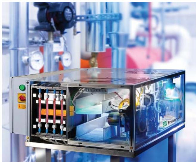
Online monitoring of water supply pipes: The biological broadband sensor AquaBioTox reacts immediately to toxic substances in water. © Fraunhofer IOSB | Picture in color and printing quality: [www.fraunhofer.de/en/press](http://www.fraunhofer.de/en/press)
