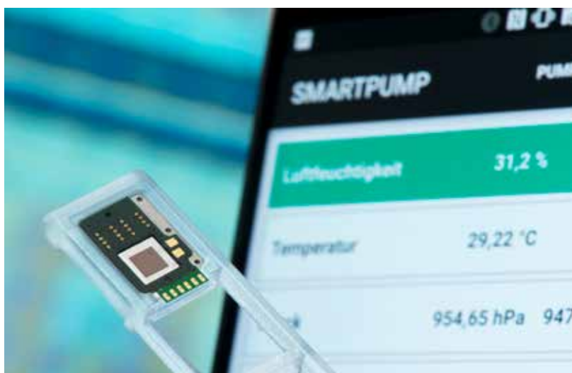
The world's smallest micromembrane pump measures just 25 square millimeters. © Fraunhofer EMFT | Picture in color and printing quality: www.fraunhofer.de/en/press
