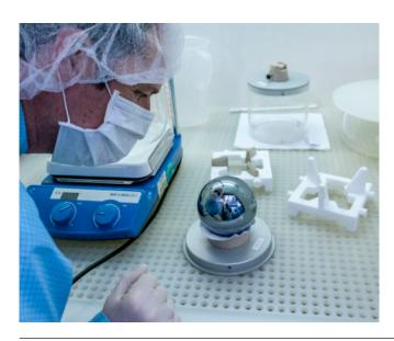
The silicon sphere to be coated must be handled like a raw egg. On the right in the picture: one of the three-point mounts. © Fraunhofer IST | Image in color and print quality: www.fraunhofer.de/ presse
