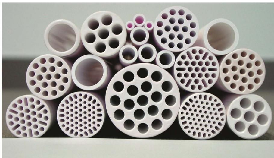
Ceramic membranes by the Fraunhofer Institute for Ceramic Technologies and Systems IKTS. © Fraunhofer IKTS | Images in color and print quality: [www.fraunhofer.de/press/research-news](http://www.fraunhofer.de/press/research-news)
