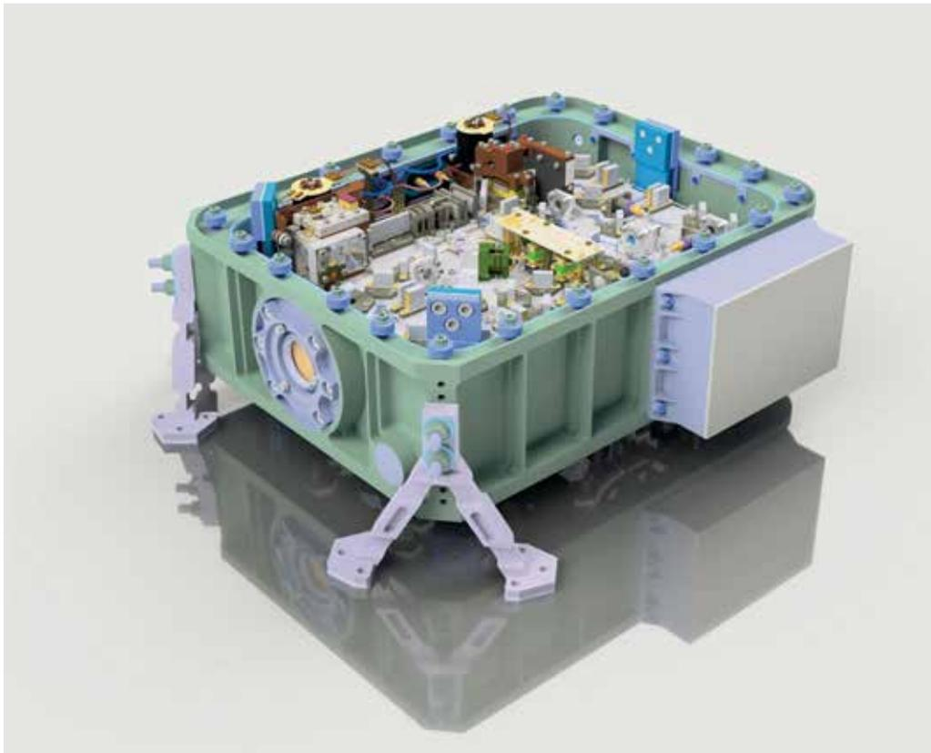
The LiDAR system for the MERLIN mission incorporates all components from the pump laser to the frequency conversion in a particularly compact design suitable for space operation. © Fraunhofer ILT, Aachen. | Picture in color and printing quality: [www.fraunhofer.de/en/press](http://www.fraunhofer.de/en/press)
