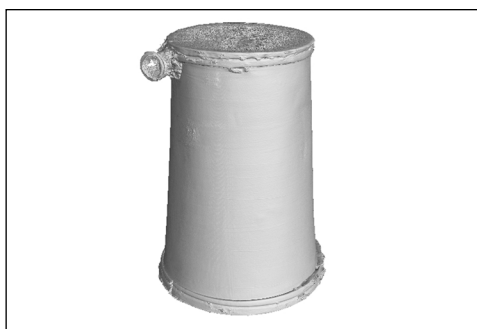
CT scan of a box-valve trumpet, viewed from the exterior © Fraunhofer EZRT | Picture in color and printing quality: www.fraunhofer.de/en/press
