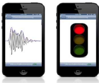
Ultrasound measurement data is transmitted to a smartphone, where it is analysed to determine a person's age (illustration). © Fraunhofer IBMT | Picture in color and printing quality: www.fraunhofer.de/en/press
