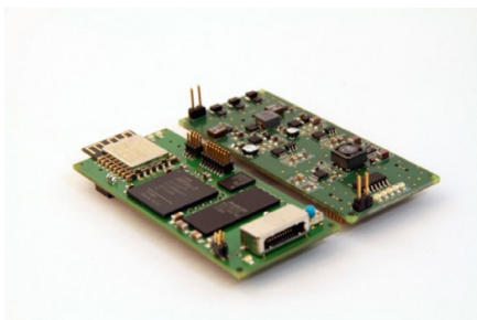
Measurement circuits on the left, power supply on the right: Fraunhofer technological excellence is at the heart of the PRIMSA portable test system. © Fraunhofer IBMT | Picture in color and printing quality: www.fraunhofer.de/en/press
