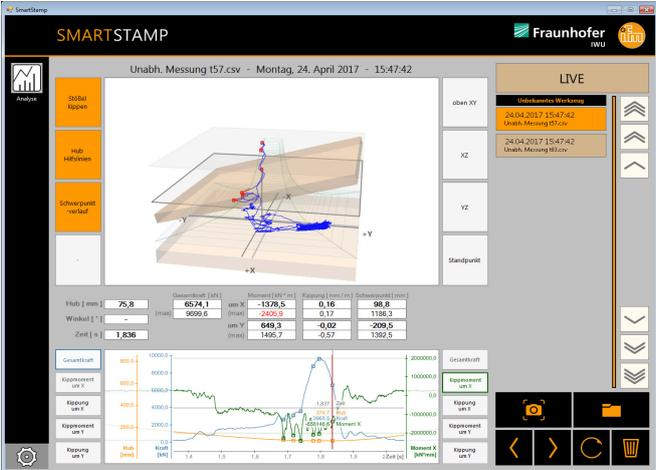
Smart Stamp: a virtual twin of the actual forming press determines the degree of ram tilt. © Fraunhofer IWU | Image in color and print quality: [www.fraunhofer.de/en/press](http://www.fraunhofer.de/en/press).
