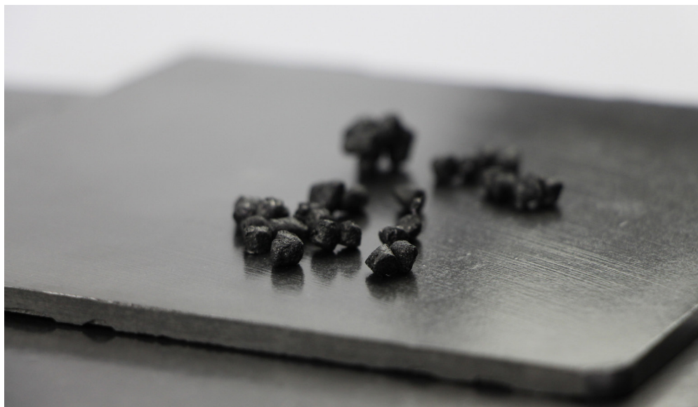
The Fraunhofer ICT uses recycled, small chopped carbon fibers (top) to produce bipolar plates (bottom) for batteries and fuel cells. © Fraunhofer IDMT | Picture in color and printing quality: www.fraunhofer.de/en/press
