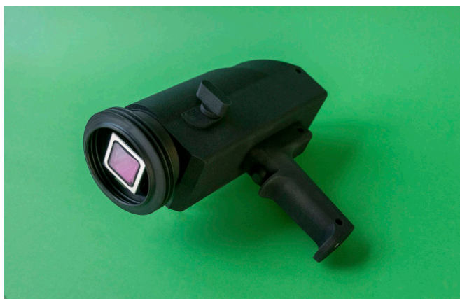
Demonstrator of a mobile measuring gun with luminescent polymeric carrier. (Fraunhofer IST / Falko Oldenburg)
