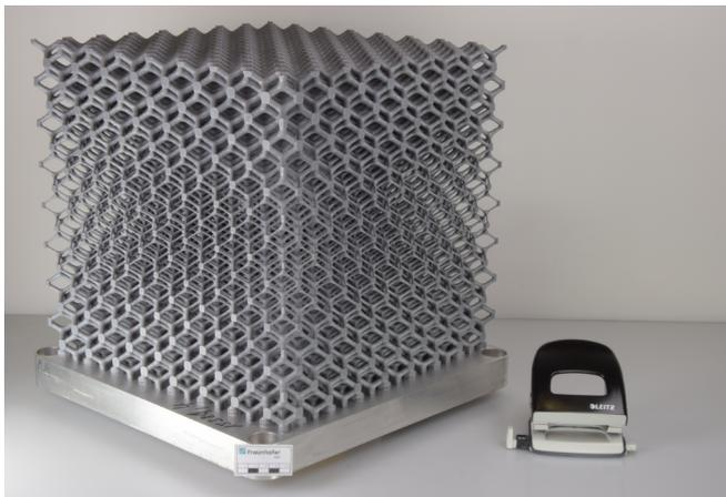
**Lattice cube with edge length of 40 centimeters, one of the largest metal structures manufactured using selective laser melting (SLM). © Fraunhofer EMI | Picture in color and printing quality: [www.fraunhofer.de/en/press](http://www.fraunhofer.de/en/press)**
