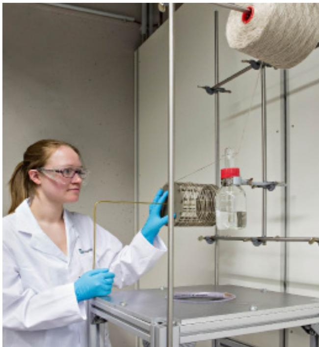
**To make the natural fibers more resistant, the roving is impregnated with monomers: the polymerization then proceeds within the yarn.**
