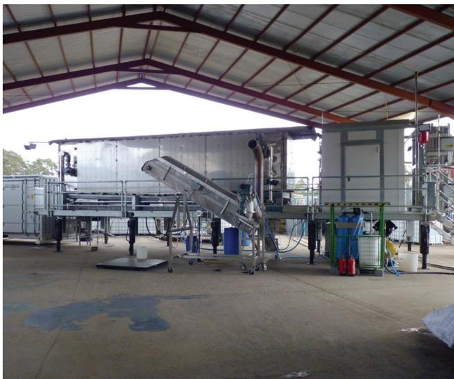
The pilot facility consists of a container with a storage bin and energy center, as well as of a frame that houses the drying and torrefaction reactors, the attachment for extracting solids and the condensers. © Fraunhofer IGB | Picture in color and printing quality: [www.fraunhofer.de/en/press](http://www.fraunhofer.de/en/press)
