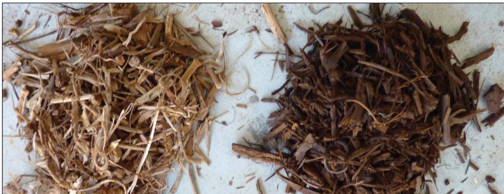
The project partner in Spain is investigating the torrefaction of various lignocellulosic substrates, including pruning (left untreated, right torrefied). © Fraunhofer IGB | Picture in color and printing quality: [www.fraunhofer.de/en/press](http://www.fraunhofer.de/en/press)
