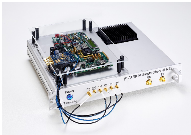
Picture 2: Single-channel version of the ATRIUM radar target simulator.
