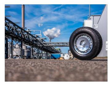
Initial testing of tires made from the nature-identical, biomimetic synthetic rubber BISYKA shows that they achieve around 30 to 50 percent less abrasion compared to natural rubber tires.
