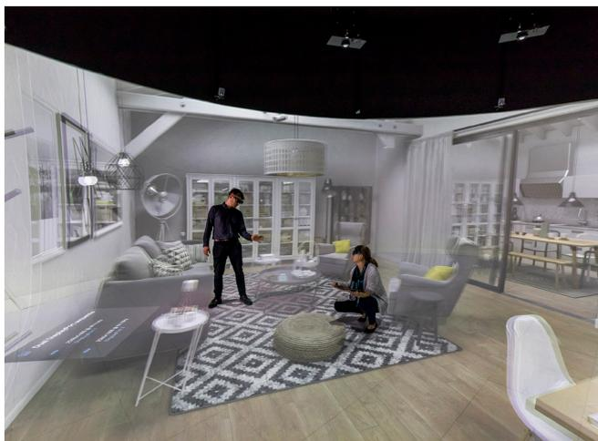
The stereoscopic projection system makes it possible to perceive virtual worlds in the Elbedome in three dimensions. Holographic representation gives users the sense of being in the midst of the projected images. © Fraunhofer IFF | Picture in color and printing quality: [www.fraunhofer.de/en/press](http://www.fraunhofer.de/en/press)
