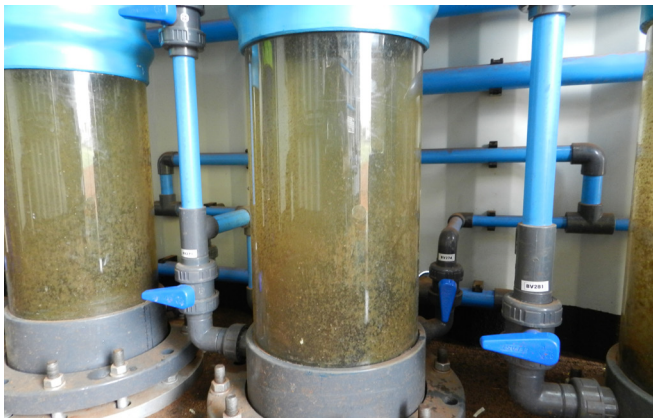
Coagulation and flocculation columns for purifying the river water. © Fraunhofer IST | Picture in color and printing quality: www.fraunhofer.de/en/press
