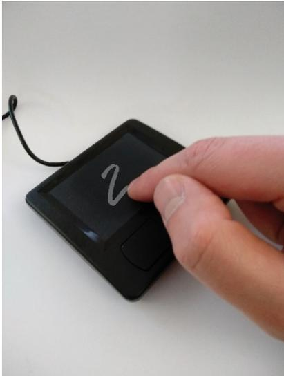
**Picture 1: AlfES demonstrator for handwriting recognition. Numbers written by hand on the PS/2 touchpad are identified and output by the microcontroller.**
