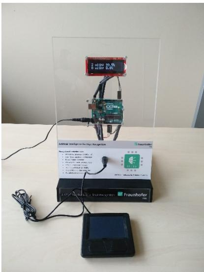
**Picture 2: AlfES demonstrator for handwriting recognition. All functions have been integrated on the Arduino UNO, which reads the sensor values of the touchpad, performs number recognition and outputs the result to the display.**
