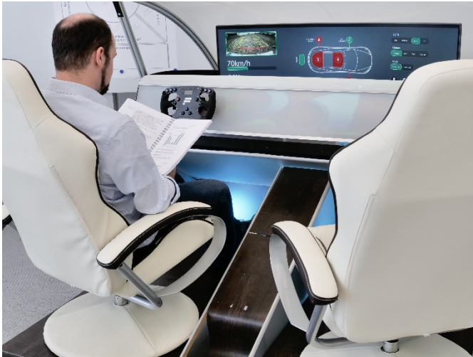
Picture 1: Fraunhofer IAO's Mobility Innovation Lab showcases the mobility of the future with a futuristic interior that features a modular dashboard, windows made of switchable glass, reclining seats, fold-out tables and a pull-out monitor.
