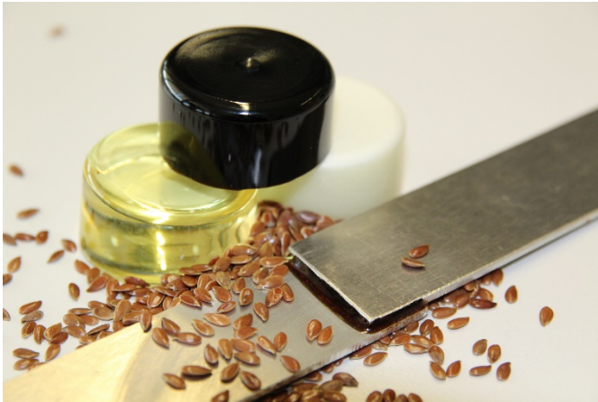
Picture 1: Two metal parts joined using the new, sustainably produced adhesive. Behind them: three pots containing the ingredients of the adhesive – the liquid hardener (yellow), the paste hardener (white) and the lignin organic solvent (black).
