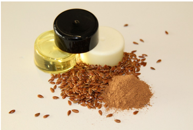
Picture 2: Powdered lignin and linseed. Behind them: three pots containing the ingredients of the adhesive – the liquid hardener (yellow), the paste hardener (white) and the lignin organic solvent (black).
