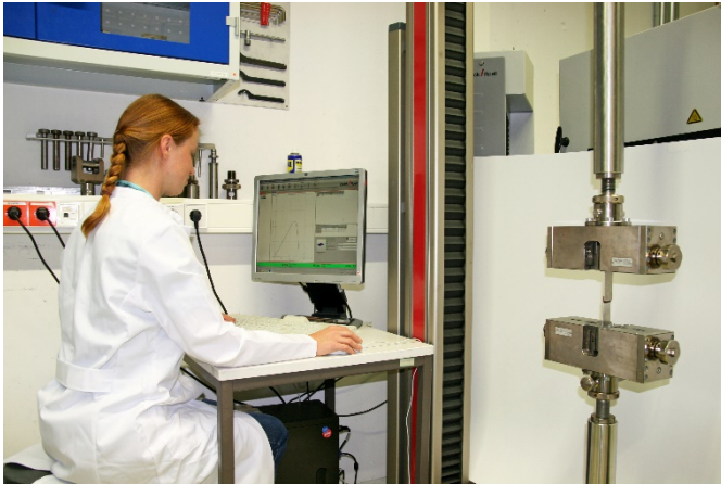
Picture 3: Assessing the measurement curve and determining the tensile shear strength.
