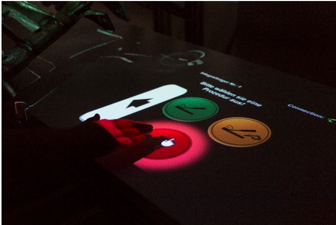
Picture 3: An augmented hand gesture-based user interface is projected onto the component and workbench, where it serves to control the robot and the inspection procedure.
