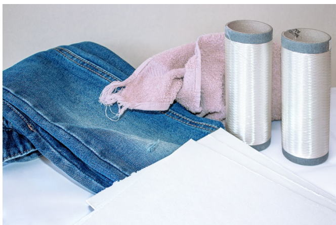
Picture 1: Wound onto a spool, the viscose filament yarn was spun from recycled cotton provided in form of cellulose sheets. Researchers at the Fraunhofer IAP have found a way to turn cotton clothes such as jeans into new high-quality garments rather than lowly cleaning rags.
