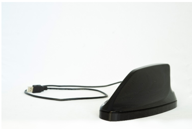
Picture 1: Teaching cars to hear: a modified roof fin for testing acoustic sensors for the capture of external noise.
