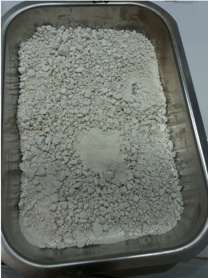
Picture 1: Recycled phosphate from sewage sludge ash, obtained via the P-bac process.
