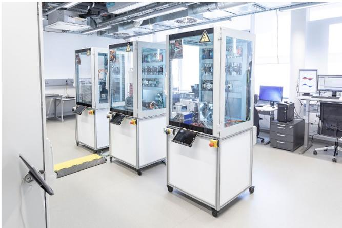
**Picture 1: The DC Laboratory at Fraunhofer IPA tests components for converting production plants to direct current.**
