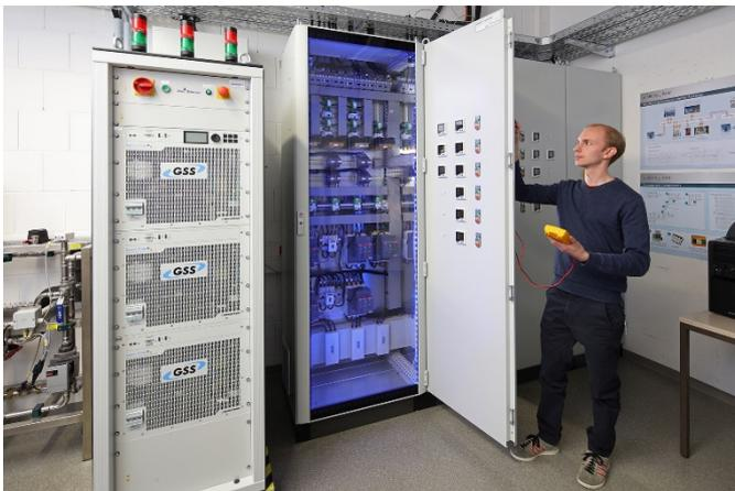
**Picture 3: Work on the main distribution neutral unit for the DC test grid at Fraunhofer IISB.**
