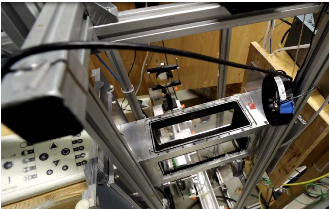
Picture 2: Tests in the wind tunnel at AIRBUS showed that the ice falls off the structured surface by itself after a defined time.
