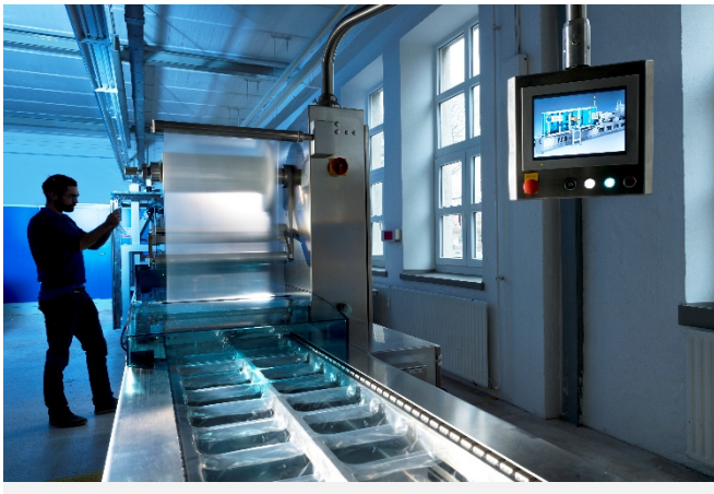
Fig. 2: Demonstrator equipment at Fraunhofer IGCV – here, a thermopackaging machine – shows how plant and associated machinery can be operated on an energy-adaptive basis.
