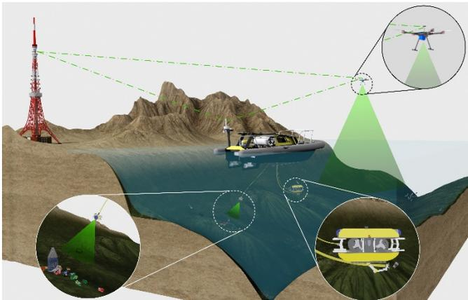
**Picture 3: Various robot vehicles are networked with one another in the SeaClear system. An autonomous or remote-controlled mother ship (UPS) on the surface is supported by two underwater robots (ROV) and a flight drone (UAV).**
