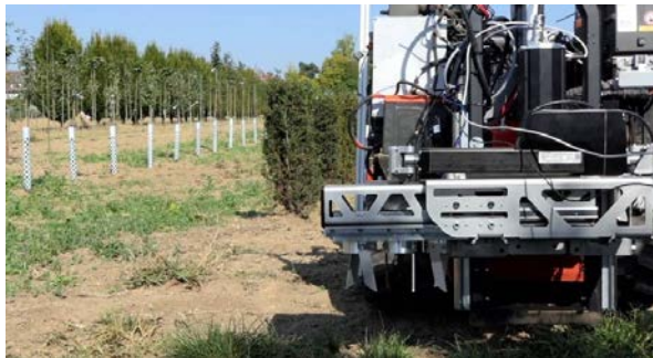
Fig. 2 The manipulator also moves in the gaps between the crop rows and removes any weeds here using the rotary harrows. © Federal Office of Agriculture and Food/Fraunhofer
