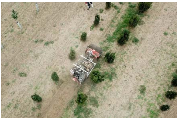
Fig. 3 The autonomous caterpillar vehicle, AMU-Bot, drives between the rows in the tree nursery and removes any weeds. © Federal Office of Agriculture and Food/Fraunhofer
