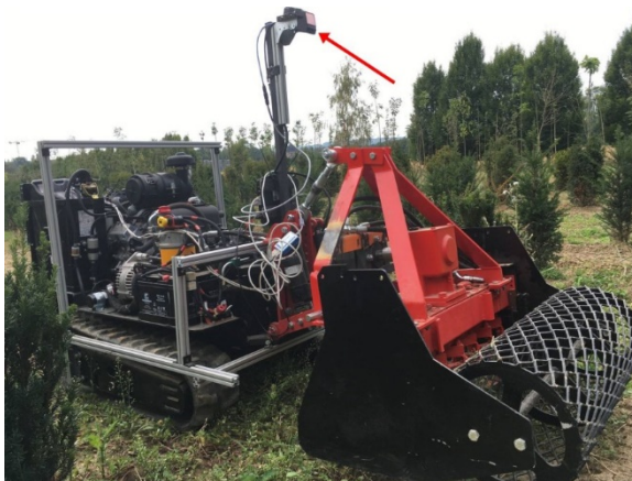
Fig. 1 The LiDAR scanner (red arrow) installed in AMU-Bot continuously emits laser pulses as the vehicle moves, which the system uses to determine the position of the crop rows. © Federal Office of Agriculture and Food/Fraunhofer
