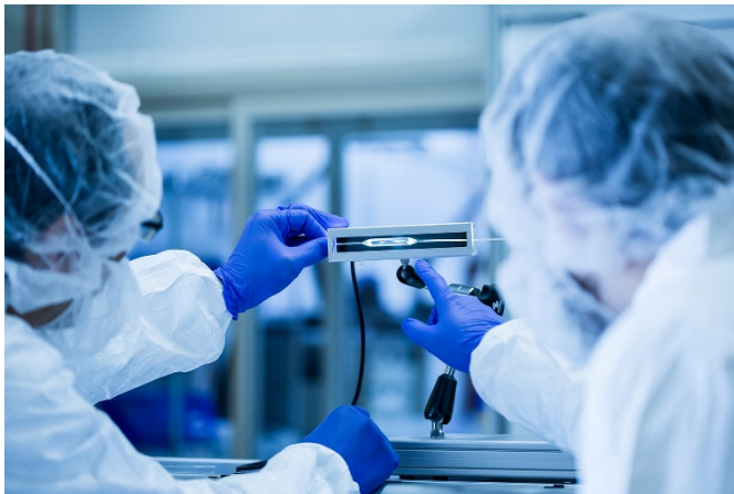
Picture 1 Optical inspection of a balloon catheter
