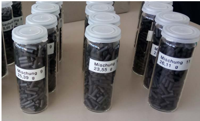
Fig. 1 The activated carbon composite from Fraunhofer has an electrical conductivity three times that of conventional granular activated carbon.
