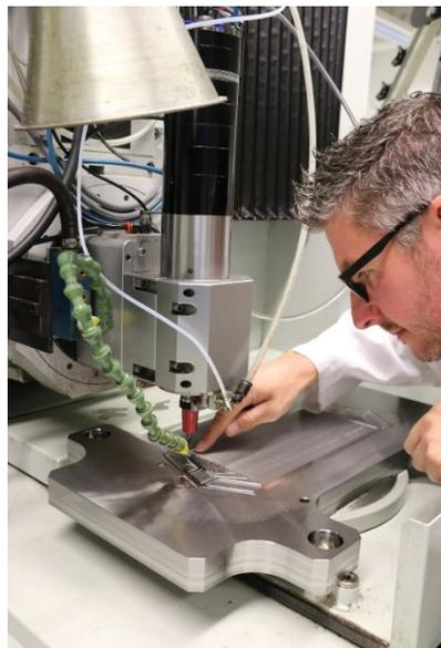
**Fig. 2 Udo Eckert, Group Leader Microsystems Manufacturing & Technical from the Functional Surfaces and Micromanufacturing department at Fraunhofer IWU, tests the finishing of a milled tool to be used in bipolar plate production for fuel cells at the micromachining center of Fraunhofer IWU.**
