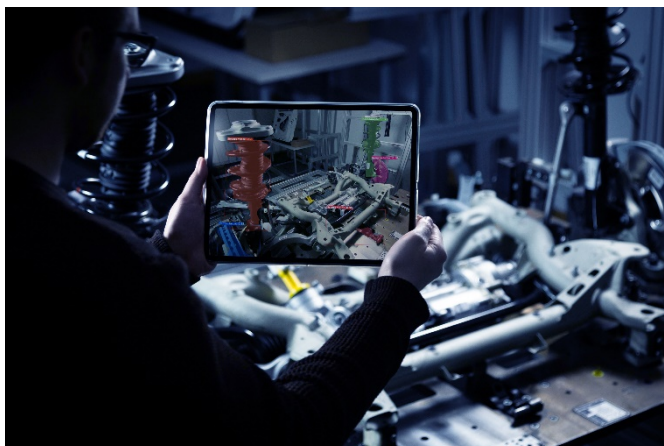
Picture 1 MARQUIS software recognizes both the component itself, and also any discrepancies from the target dimensions.
