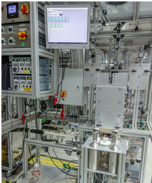
Picture 3 Catalytic converter test rig: This is used to test all the functions of a catalytic converter, as well as its efficiency in waste gas purification. Fraunhofer IMM has a total of nine test rigs.
